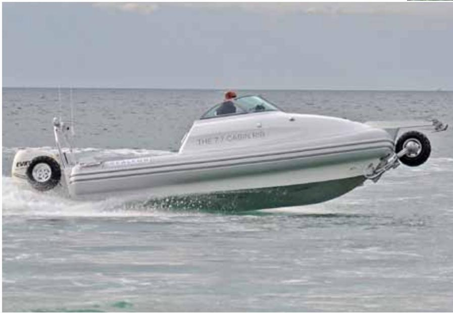
Kiwi company Sealegs has built a solid reputation for its amphibious RIBs – boats that drive over land and straight into the water. Once floating, simply retract the wheels and you've got a high-performance powerboat.
