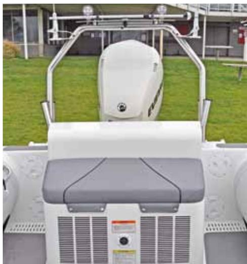
*Right: The engine pod allows extra room for housing the engine that powers the hydraulics – a 24hp Honda.*
